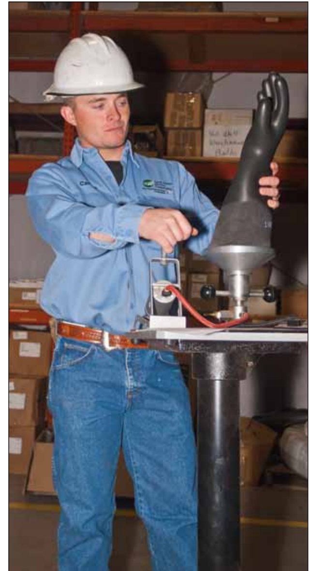
Carlyle Stokes checks his rubber gloves for leaks and damage. Linemen check their gloves and other rubber goods daily.
